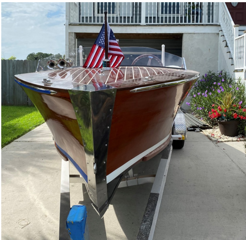
Photograph 5. About two months prior to launch, the hull polishing was completed. The hull and decks have 15 coats of marine varnish, which was then polished with 1000, 1200, 1500 and 2000 grit sandpaper to bring out the luster.
